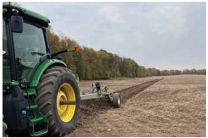
MIC with deep chisels inserted to 24 inches can be drawn by a 240 horse power unit at a swift walking speed.
