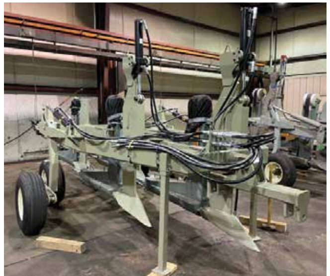
Two Membrane Installation Chisels (MIC's) at the SWRT Solutions shop awaiting field season
