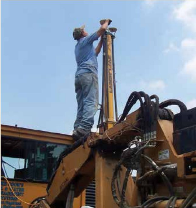
LICA member Mike Cook makes adjustments to the Spectra Analog mast during field trials for the “Pipe” software program.
