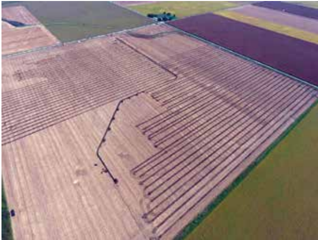
Drone image of fall 2016 drainage design. Image courtesy of Waterborne Environmental.
